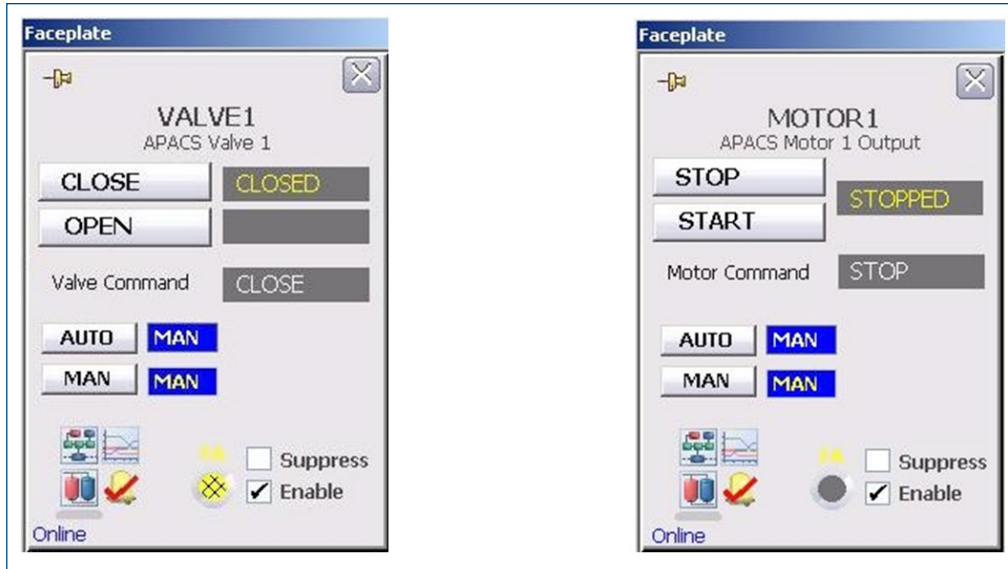
Figure 5. DeltaV Connect Solution for Moore Systems VALVE & MOTOR faceplates.
